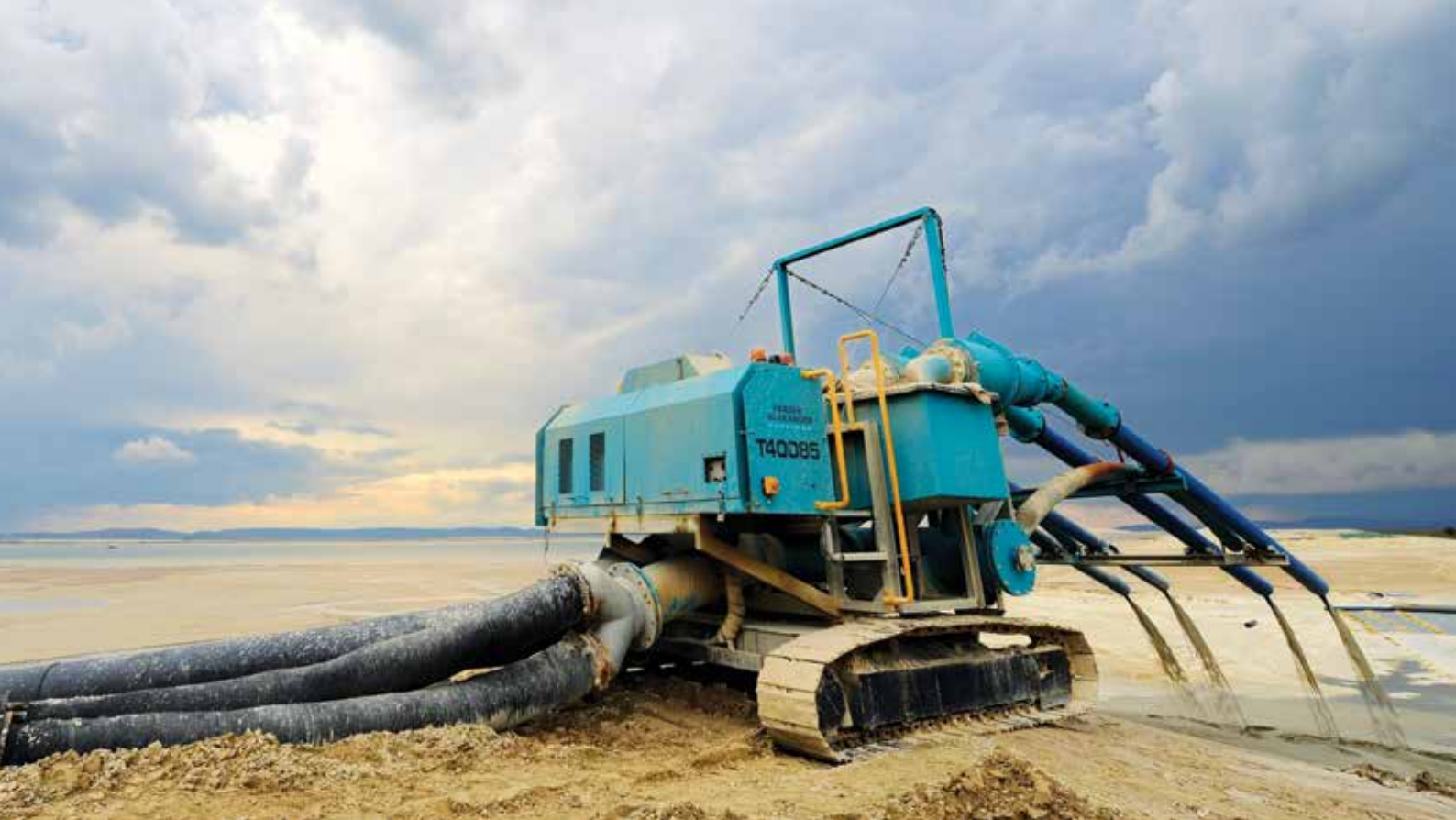
Above: A self-propelled cyclone unit depositing discarded tailings on the BTF
